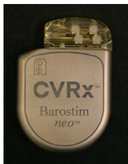
Figure 2: Implantable Pulse Generator
